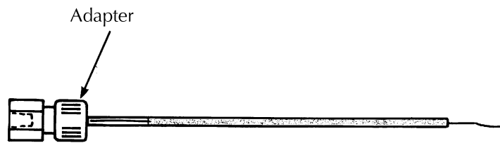
Figure 15. Inserting the top of the Analytical Tube Gel into the adapter
