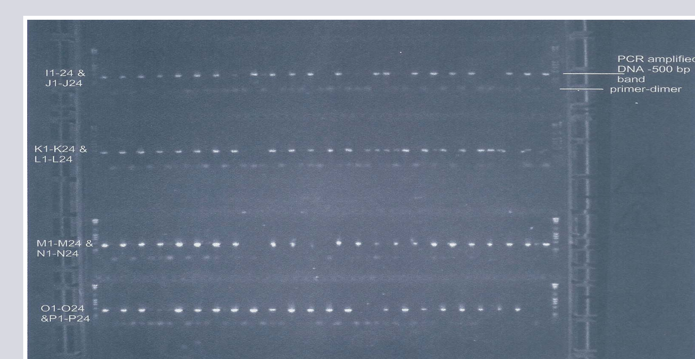
Figure 2: Bottom half of PCR plate 1 (source plate had DNA and water in alternating wells)
