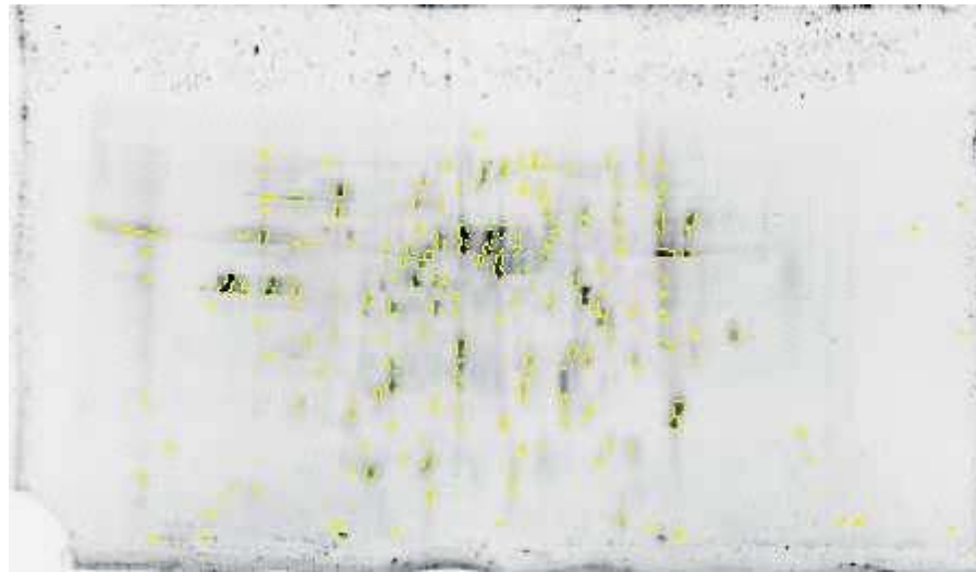
Figure 2: Criterion Medium Format gel (13 x 9 cm) with 11 cm IPG strip
